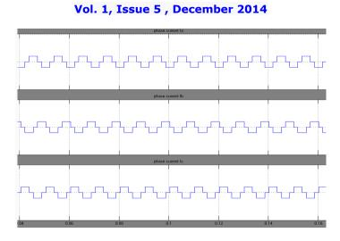
Fig 6. Phase current wave forms of Four-switch inverter fed BLDC motor
