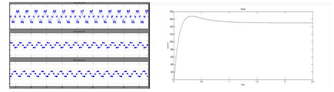
Fig 13.Phase currents using fuzzy controller Fig 14.Speed profile of the drive for fuzzy controller
