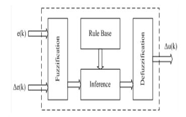
Fig 8 Structure of Fuzzy Logic Controller
