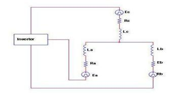
Fig 1.Equivalent circuit of BLDC motor
