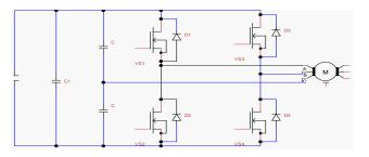
Fig 3.Four-switch three-phase inverter
