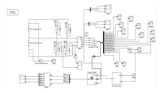
Fig 12 Simulink diagram of four-switch Inverter fed BLDC motor using fuzzy logic
