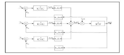
Fig 2.Transfer function model of BLDC motor
