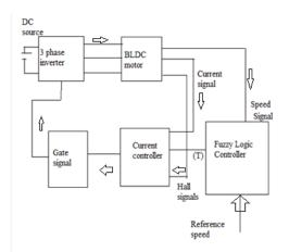
Fig 7.Proposed BLDC motor with Fuzzy Logic Controller
