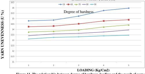
Figure 11. The relationship between degree of hardness, loading and the result of yarn unevenness (U %) (Diameter : 33x17, 9.8Tex)
