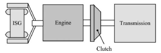
Fig -2 – ISG layout in passenger car [9]
