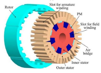
Fig -3 – Permanent Magnet Hybrid Brushless system [9]
