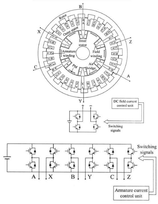
Fig -4 – Layout of the complete Hybrid ISG system [9]
