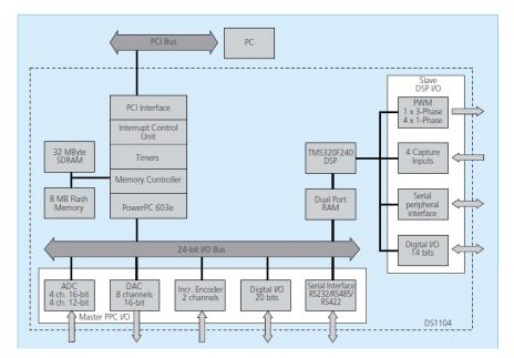
Fig -7 – Block diagram of dSPACE 1104 module
