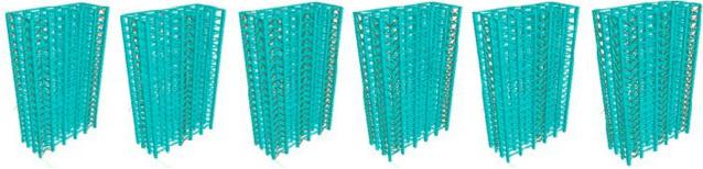
Fig 5: Chevron bracings and V bracings at corner, center and alternate locations
