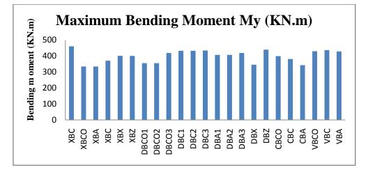
Fig 6.Maximum Bending Moment My (KN.m) for different Bracing Systems
