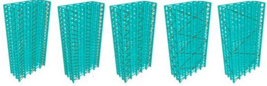
Fig 4: Different Locations of diagonal bracings
