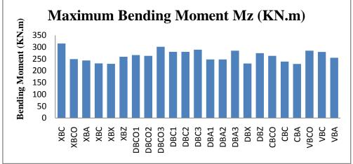
Fig 7.Maximum Bending Moment Mz (KN.m) for different Bracing Systems
