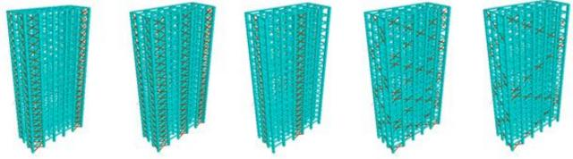
Fig 2: Different Locations of X bracings at Corner, Alternate, Centre, Configuration X and Configuration Zigzag
