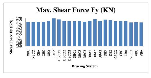
Fig 8. Maximum Shear Force Fy (KN) for different Bracing Systems
