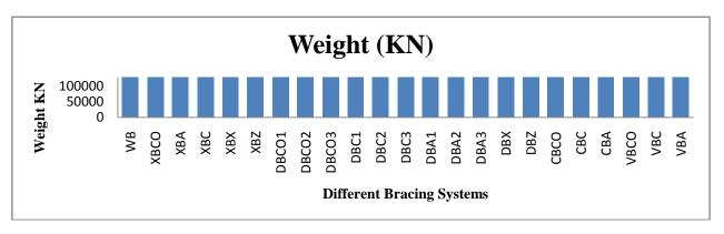
Fig 10.Weight of Structure with different bracing systems
