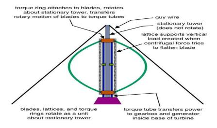
Figure 3: High Mechanical Efficiency Centrifugally Stable Darrieus Turbine VAWT's Used in Practice:
