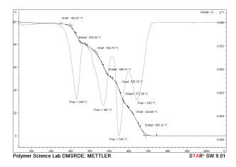
Fig. 2. TGA of 400 mg Carbon Black/ ml PU Nano-composite
