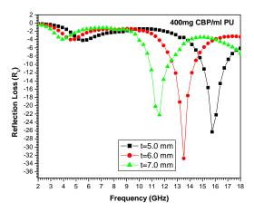
Fig. 4. Reflection loss (R<sub>L</sub>, dB) vs. frequency (GHz) for t= 5, 6 and 7 mm
