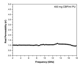
Fig. 3. Variation of Real permeability (μ') with frequency (GHz) of CBP/PU Nano-composite
