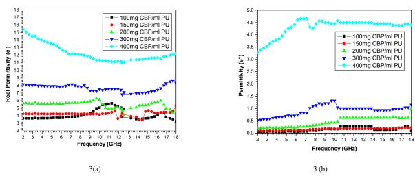
Fig. 2. Variation of the (a) Dielectric constant ( $\epsilon$ ') with frequency (GHz) (b) Dielectric Loss ( $\epsilon$ '') with frequency (GHz) of CBP/PU Nano-composite
