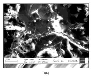
Fig. 1. Scanning Electron Micrographs (a) Carbon Black Powder (CBP) (b) SEM of Poly Urethane (PU)
