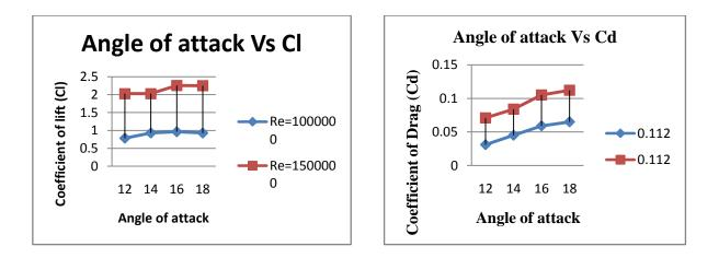
From above graph that as much as angle of attack is increased the coefficient of lift (Cl) is also increased hence lift is increase. But one condition comes when lift cannot be increased further and goes to reduced continuously. This reduction due to the generation of adverse pressure gradient at the trailing edge.
