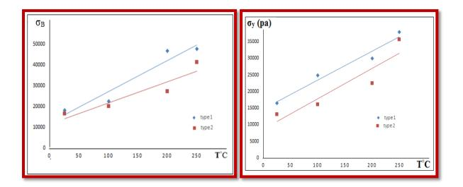
Figure (4) shows stress at break as a function for heat treatment in different temperatures PTFE.
