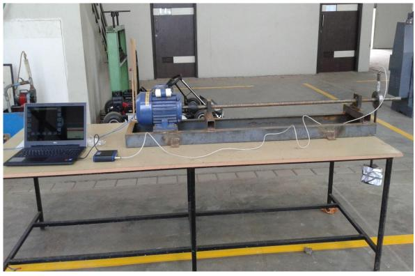
Fig. 1. Experimental Setup: Test rig of Defect detection analysis of Deep Groove Ball bearing
