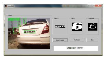
Figure 12. GUI model for license plate recognition system
