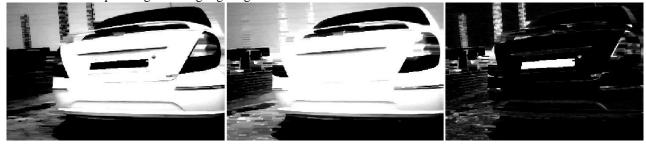
(a) (b) (c) Figure 4 (a) Opening (b) Closing of gray scale image & (c) Difference of opening and closing image
