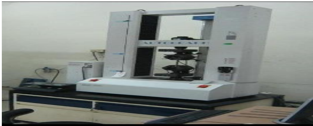
Figure.5.Loading of Specimen in UTN 40 Models UTM
