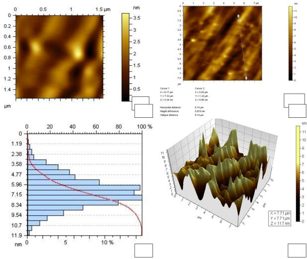
Fig.2. Distribution of Ni clusters on Si surface (AFM). a) — silicon sample excluding Ni clusters, b) — annealing duration 1 hour, v) — annealing duration 2 hours, d) — annealing duration3hours, e) –integral and differential distribution of Ni clusters in silicon, g) - distribution of Ni clusters in silicon.
