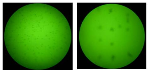
Fig. 1. Distribution of clusters of Ni atoms on silicon sample surface (INFRA-I – infrared microscope photo depict)
