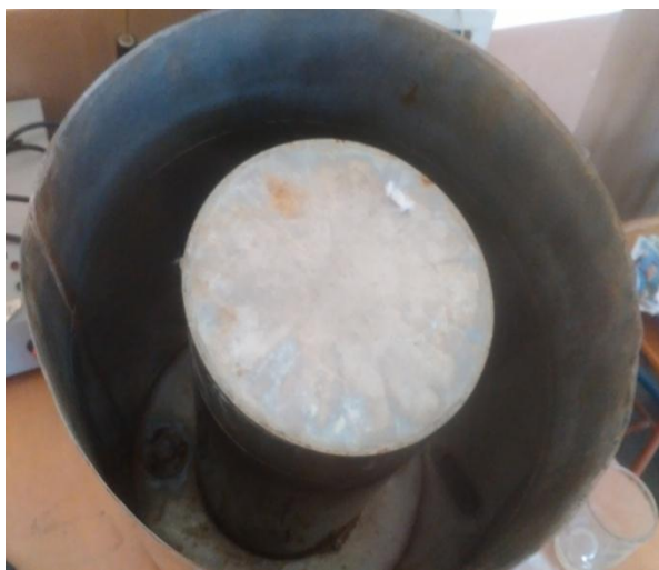
Figure 4.2 – bomb calorimeter jacket after removing back cover.
