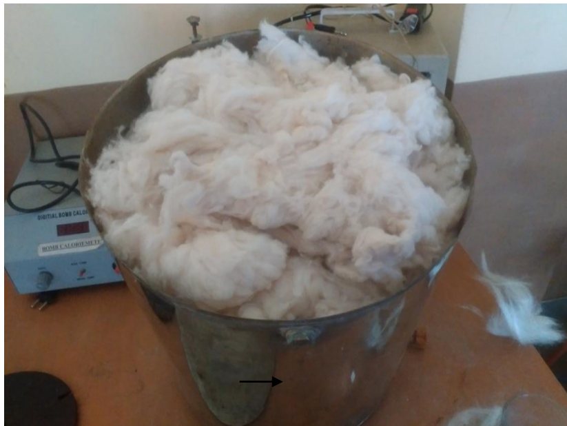
Figure 4.5: Bomb calorimeter jacket filled with cotton wool
