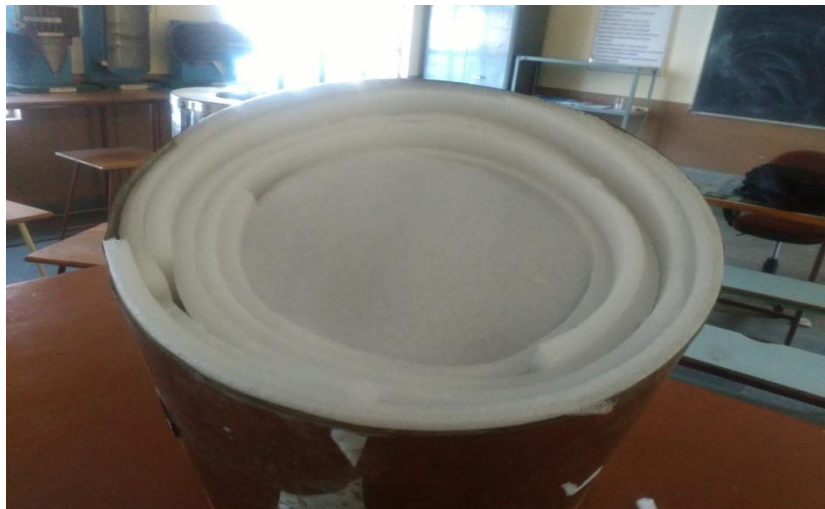
Figure 4.7: Bomb calorimeter jacket filled with cotton wool
