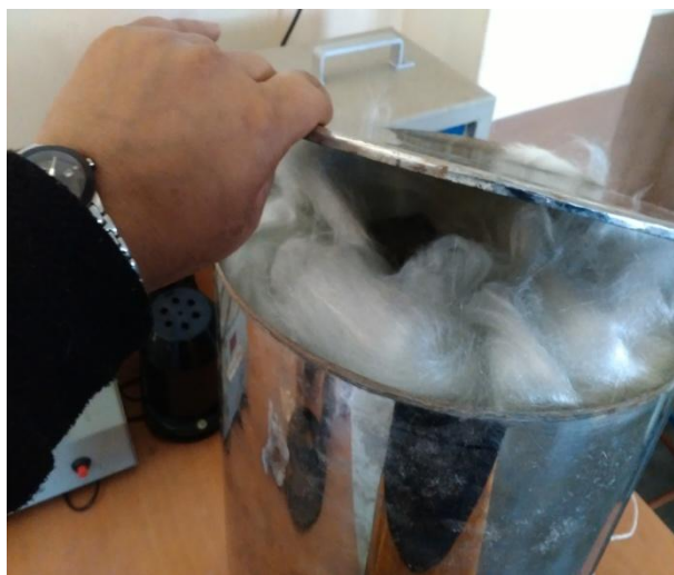
Figure 4.3 – bomb calorimeter jacket filling with glass wool
