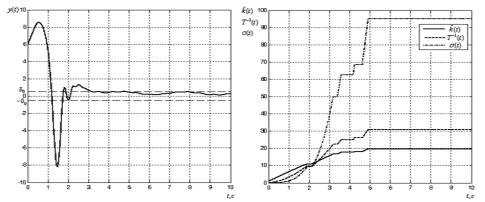
Figure 1 - The transients in a control system (40), (41), (33), (9) and the variable adaptive controller tuning parameters
