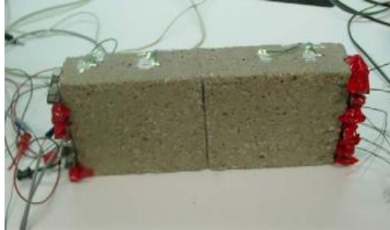
Fig6. A small concrete block post-tensioned with SMA wires
