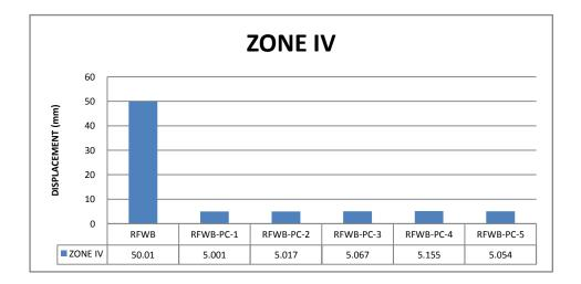
Comparison of displacement for seismic zone IV
