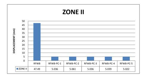
Comparison of displacements for seismic zone II
