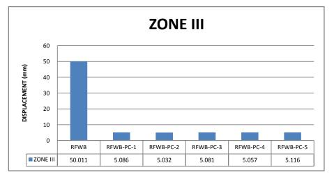
Comparison of displacements for seismic zone III
