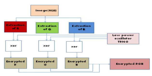
Fig. 2: proposed image Encryption Architecture
