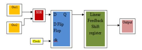
Fig. 3: Architecture of Proposed RNG
