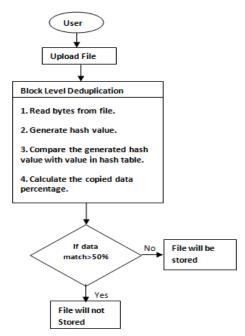
Fig 4: Block Level deduplication Process
