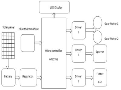
Fig. Block diagram
