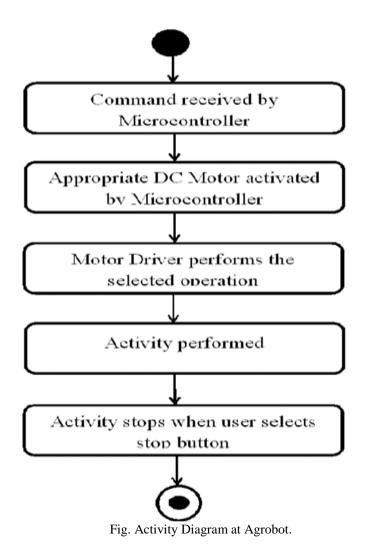
As illustrated in the figure, the Bluetooth receiver at the Agrobot receives the ID (Identifier) passes by the user and passes the message on to the Microcontroller. Appropriate DC Motor that has to be activated is deduced by the Microcontroller. The Motor Driver activates the corresponding motor and performs the selected operation. The Agrobot now waits for the stop signal to be received in order to stop functioning.
