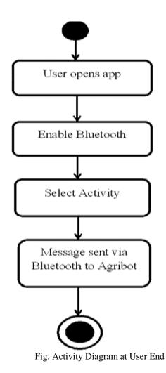
The figure shows the activity diagram at user end. When the user opens the application, a message requesting Bluetooth to be enabled appears. Once the Bluetooth is switched on and the Agrobot is paired a list of activities appears. The user selects the desired activity and the id corresponding to the activity is sent to the Agrobot via Bluetooth.
