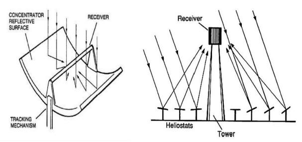
Fig. 1. Parabolic trough systemFig.2. Central Receiver Tower System
