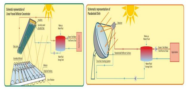
**Fig. 3.** Schematic representation of Linear **Fig. 4.** Schematic representation of Parabolic Dish Reflector [9] Fresnel Reflector Concentrator [8].
