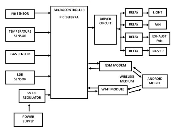
Figure 1: Block Diagram of Home Automation
