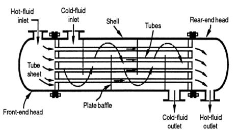
Fig.3.1 Shell-and-tube exchanger [10]
