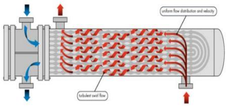
Fig.4.1 Twisted tube heat exchanger [9]
