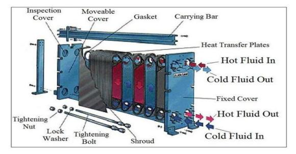
Fig.3.2 Plate heat exchangers [11]
