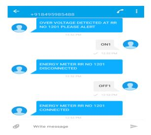
Fig. 5.3 Over voltage detection and control
