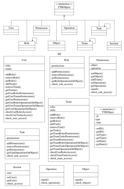
Figure 1: TT-RBAC core classes: (a) inheritances; (b) definitions
