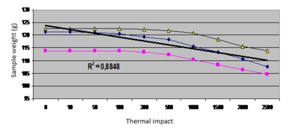
The schedule of loss of weight of tested samples of building designs depending on thermal influence.
