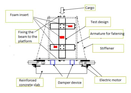
The test scheme on a seism platform of a Ferro-concrete design with special inserts from vermiculite foam.
