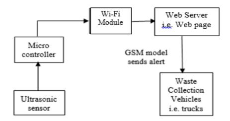
Fig. 1: Smart Waste Management System BlockDiagram
