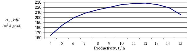
Fig.1. Changes in the volume coefficient of heat transfer  $\alpha_v$  depending on the productivity of the drying drum
