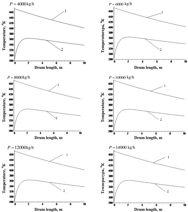
Fig.2. Changes in the temperature of the drying agent (1) and raw cotton (2) along the length of the druma
