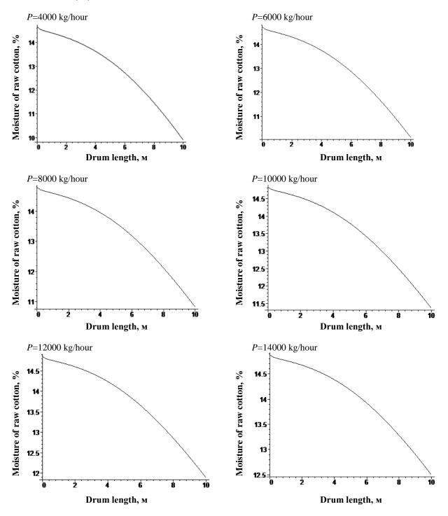
Fig.3. Changes in the moisture content of raw cotton along the length of the drying drum
