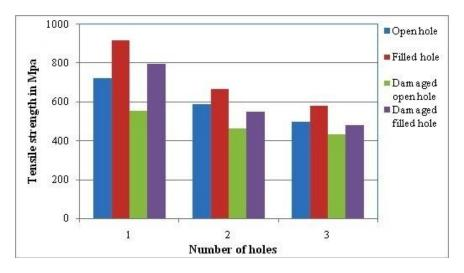
Fig 10 Analyses of tensile strength results of 1 hole, 2 holes and 3 holes in the specimens
