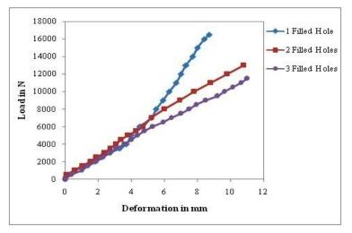
Fig 7 Load v/s deformation curve for specimens have 1 hole, 2 holes and 3 holes is placed with M6 bolt
