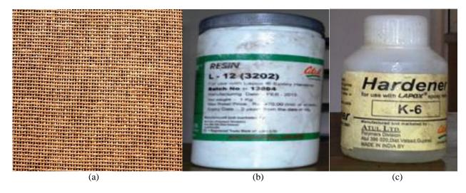
Fig.1 Raw materials used for composites: (a) jute fabric, (b) Lapox L-12 epoxy resin and (c) hardener k-6
