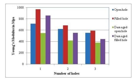
Fig 11 Analyses of modulus of elasticity results of 1 hole, 2 holes and 3 holes in the specimens.
