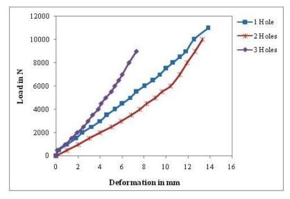
Fig 8 Load v/s deformation curve for damaged Specimens have 1 hole, 2 holes and 3 holes
