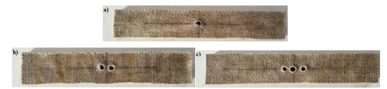
Fig 4 Number of holes in the damaged specimen along horizontal axis; (a) 1 hole, (b) 2 holes and (c) 3 holes
