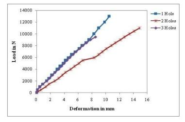
Fig 6 load v/s deformation curves for specimens have 1 hole, 2 holes and 3 holes
