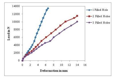
Fig 9 Load v/s deformation curve for damaged specimens have 1 hole, 2 holes and 3 holes is placed with M6 bolt
