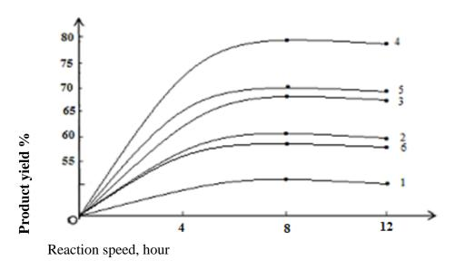
Figure 1.Dependence of the product yield on the ratio of kaolin to methyl cellulose in time.
