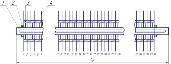
Fig. 5. Scheme of assembling a new design equipped with circular saws of the experimental unit of the saw cylinder.
