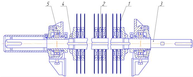
Fig.1. Design of the assembly of the saw cylinder of the fiber separating machine.
