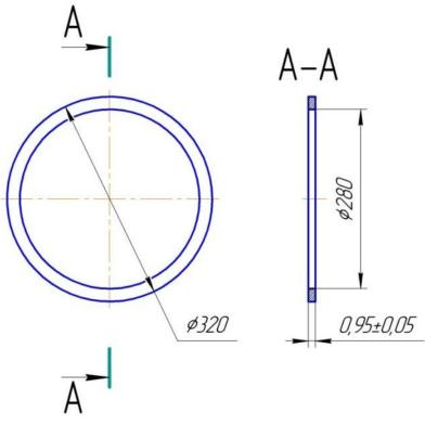
Fig. 2. Parameters of specimens-rings subjected to heat treatment.
