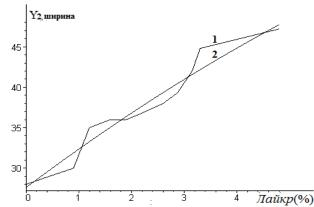
Fig.4. Graphs of the expert (curve 1) and approximating (curve 2) curves for width extensibility versus lycra in%
