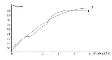
Fig.1. Graphs of the expert (curve 1) and approximating (curve 2) curves for the reverse deformation along the length of the Lycra quantity in%
