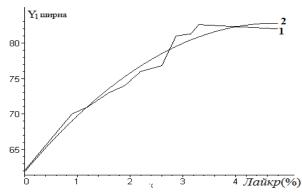
Fig. 2. Graphs of the experimental (curve 1) and approximating (curve 2) curves for the reverse deformation in width from the amount of Lycra in%
