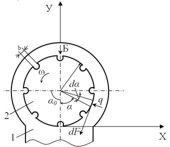
1-axis (cylinder), 2-pin (housing) Fig. 2. Calculation scheme for determining the moment of friction
