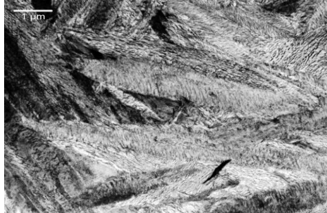
Figure 2.3. Lower bainite generated by isothermal transformation of 52100 steel at 230°C for 10 h [11].
