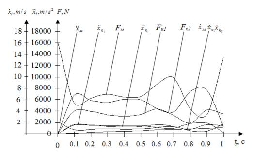
Figure 4. Pattern of change in the HUM MH-2.4 motion parameters under horizontal oscillations at  $h_w = 40 \text{ mm}$
