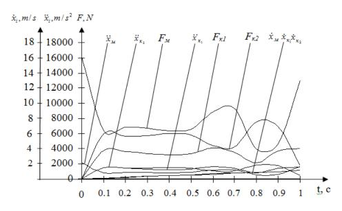
Figure.3. Pattern of change in HUM MH-2.4 motion parameters under horizontal oscillations ath<sub>w</sub>=30 mm
