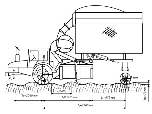
Figure. 1. Design scheme of HUM MH-2.4
