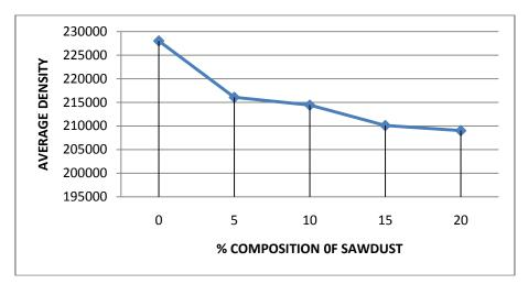
Fig. 2: Relationship between density of the specimens and sawdust content
