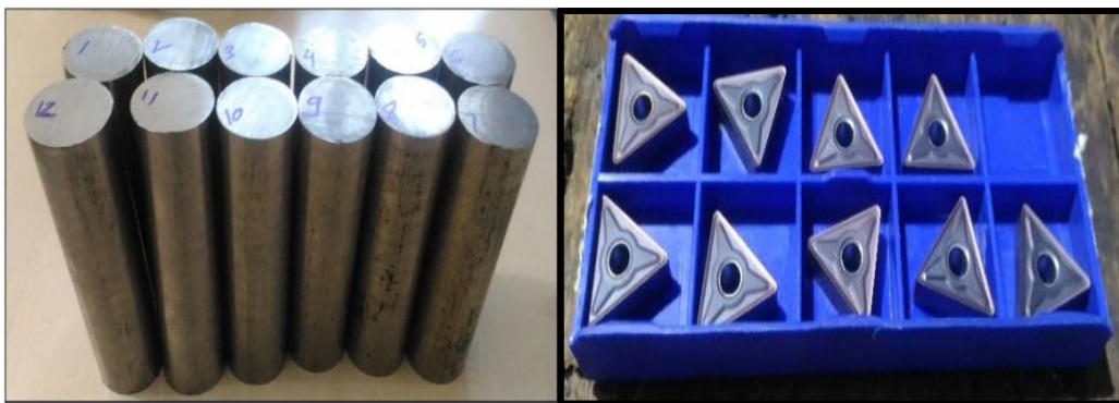
Figure No.1 - Workpiece Material AISI 316 Figure No.2- Inserts used for turning
