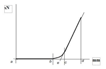
Fig.2. Diagram straightening and stretching the filaments taken out of fabric
