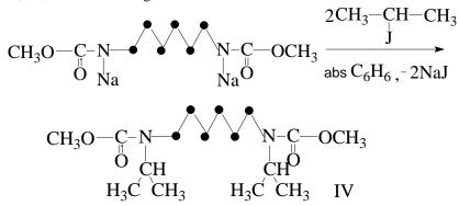
The course of the alkylation reaction exclusively on the nitrogen atom N,  $N^1$  - is explained, apparently, by the relatively easy dissociation of sodium in this atom due to the presence of carbonic groups in the neighboring. The yield of the product (IV) is 88,6 %, Mp = 157-158 °C.
