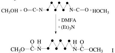
The reaction of hexamethylene diisocyanate with methanol was carried out at a molar ratio of reagents of 1: 2 at room temperature of 27-36 ° C for 3 -3,5 hours. As a result of the reaction, N, N<sup>1</sup>-hexamethylene-bis [(methanoyl) - carbamate] (I) is formed, which is a snow-white high-melting powder, difficultly soluble in water and other non-polar
