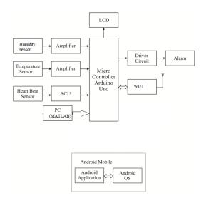
Fig.3. Block diagram of Neonate Monitoring System
