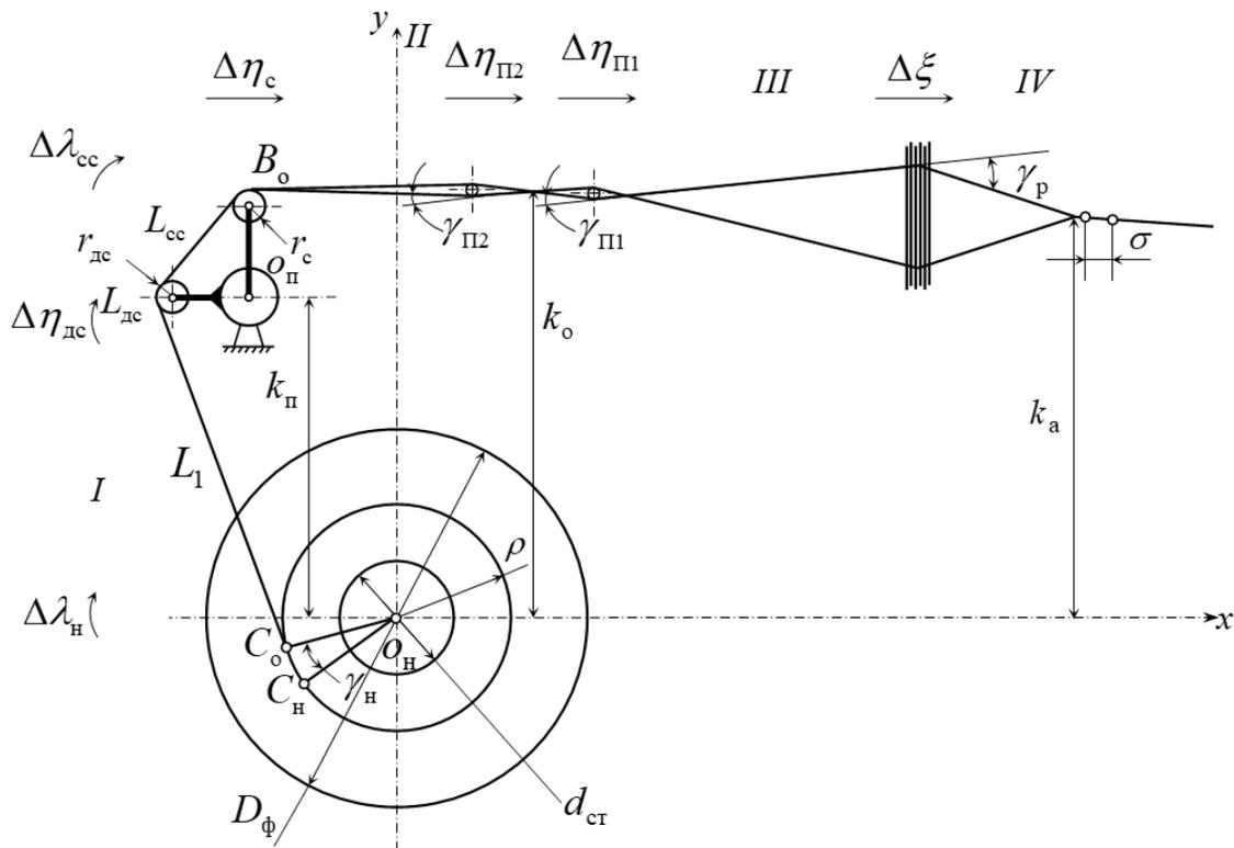
Fig 1 - Scheme of threading the warp thread on the weaving machine
