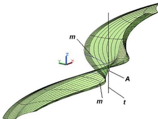
1-picture. The helical surface, its sections  $m$  and the plane  $n$ , the coordinates  $ZY$  and  $ZX$  parallel, the intersection of these parts  $t$  at point  $A$
