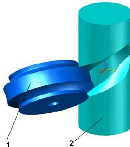
5-picture. Screw cutting (1) and cylinder forming (2) model of disc cutting
