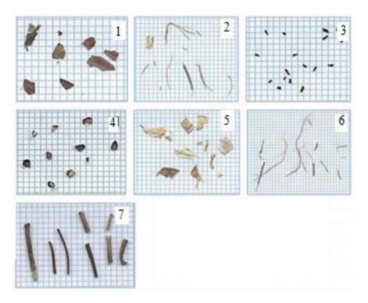
Figure 1 Classification of machine and hand picked cotton pollution 1 - leaf, 2 - stem, 3 - funiculi 4 - seed coat, 5 - shale, 6 - grass, 7 - steck.
