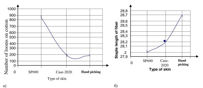
Figure 3. Graphical analysis of the indicators of cotton fiber affecting spinning.
