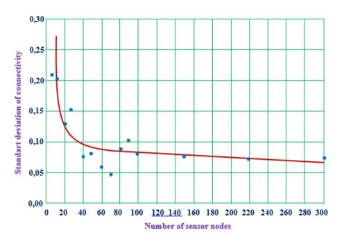
Fig. 4. Dependence of the standard deviation (SD) of the network connectivity probability on the number of network nodes
