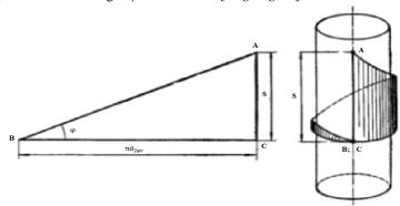
Fig 1. Formation of a helical surface
