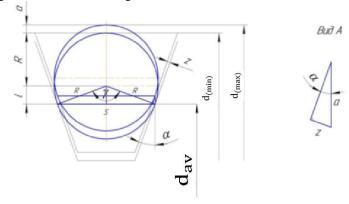
Fig.3 Determination of allowance.
