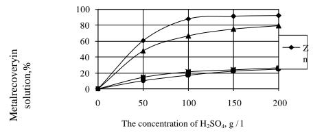
Fig. 1.The dependence of the degree of extraction of metals in solution from the concentration of acid.
