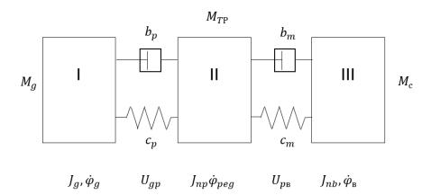
Fig. 2. Design diagram of machine unit with conveyor screw drive mechanism for transportation and cleaning of cotton lint.
