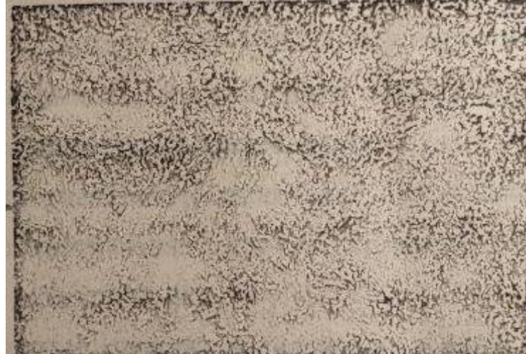
Fig. 2. Steel U8 in the delivery state.
