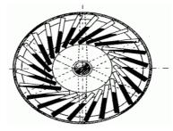
Fig.2.Bhaskara wheel with mercury in tilted vial.
