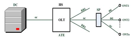
Fig 1.Model of a fragment of a rural (RTN) built on the basis of PON technology.
