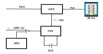
Fig 2. Organization of uninterrupted power supply at the subscriber level
