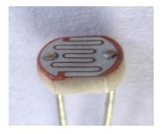
Figure 5: Optical Sensor (LDR)
