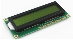
Figure 2: Liquid crystal display(16x2)
