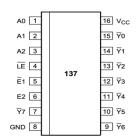
Figure 10: Pin Configuration of 74HC137
