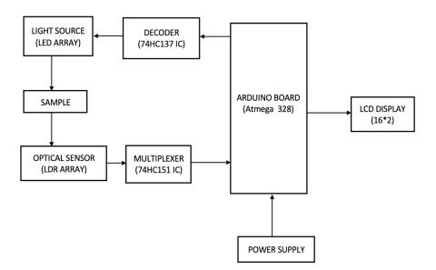
Figure 11: Block diagram
